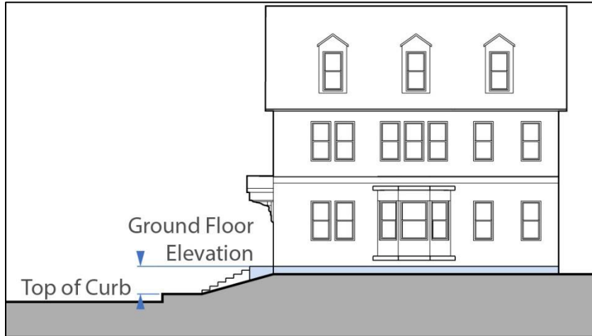
FIGURE 11: GROUND FLOOR ELEVATION
